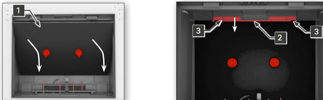
Fig.6: Back Reflective Panel Installation
