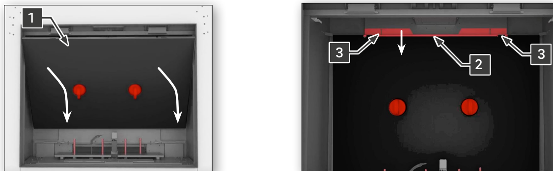
Fig.6: Back Reflective Panel Installation
