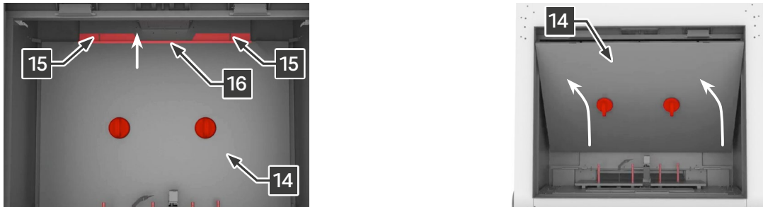
Fig.5: Back Panel Removal
